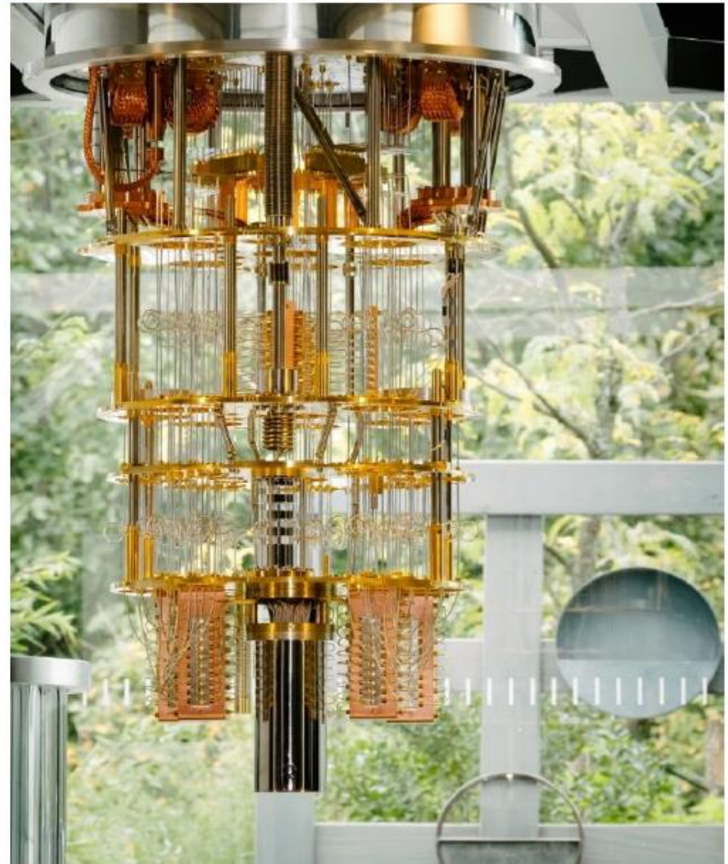
IBM 53-qubit superconductor-based quantum computer
