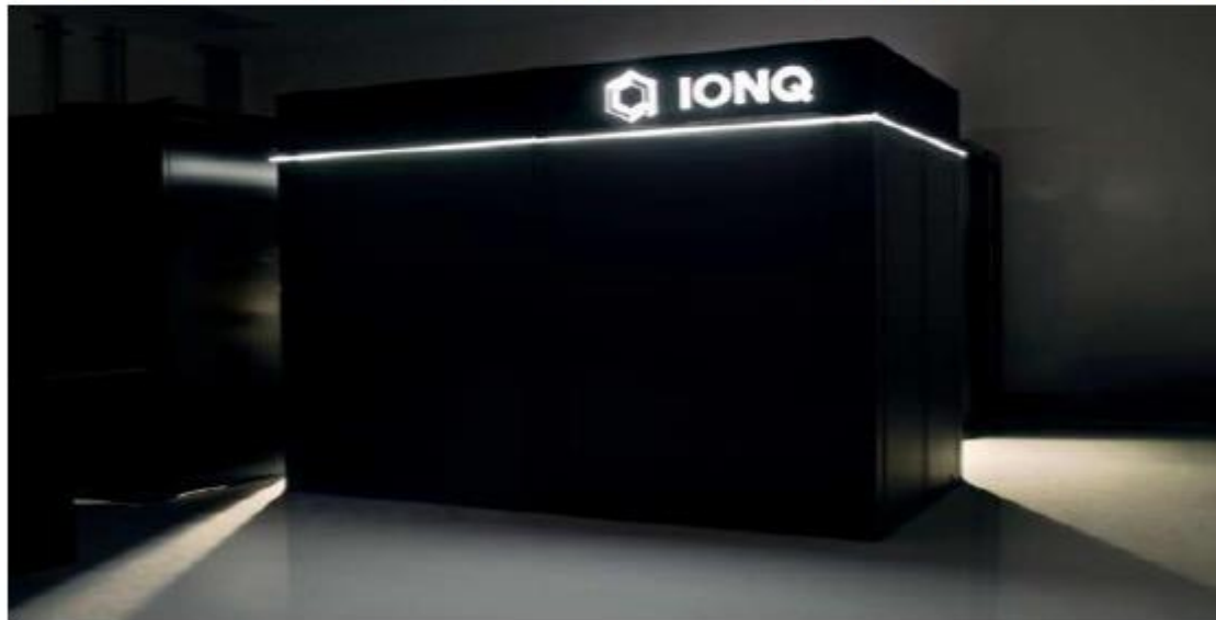
IonQ, ion-trap-based 32-qubit quantum computer
